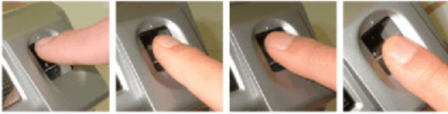
Figure 1: Improper Alignment Causes Problems
