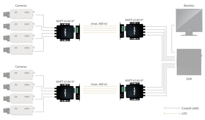
\* NVPT-414V-II allows for connection of twisted pair ended with RJ-45 connectors or for direct connection to screw terminal
