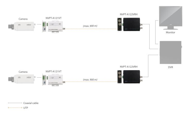
Video transmission system based on set of active transmitters and receivers NVPT-A122VR
