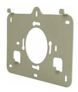
The NVE-MBRK bracket is designed for mounting a user monitor with the use of a Ø60 flush-mounted one-gang box. The one-gang box provides space for the RJ45 connector of the user monitor. The bracket allows to install the user monitor without the requirement to drill additional holes for mounting screws.
