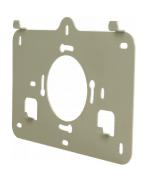
The NVE-MBRK bracket is designed for mounting a user monitor with the use of a  $\emptyset$ 60 flush-mounted one-gang box. The one-gang box provides space for the RJ45 connector of the user monitor. The bracket allows to install the user monitor without the requirement to drill additional holes for mounting screws.
