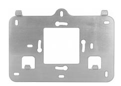
The NVE-MBRK-II bracket is designed for mounting a user monitor with the use of a Ø60 flush-mounted one-gang box. The one-gang box provides space for the RJ45 connector of the user monitor. The bracket allows to install the user monitor without the requirement to drill additional holes for mounting screws.
