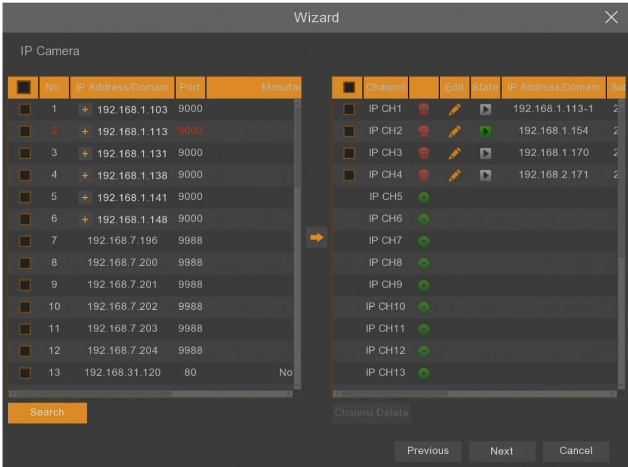
The **Search** button starts researching IP devices. The recorders IP addresses are with
