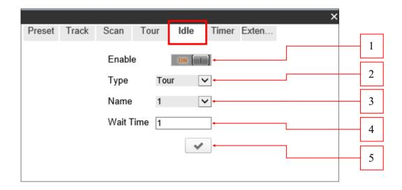
The idle function could be switched on and off by using the *on/off button* (1). When the idle function is enable, select in the *Type field* (2) the program function which is activated after the *waiting time* (4), then select the function name in the *Name field* (3). The program functions has to be programmed before.
