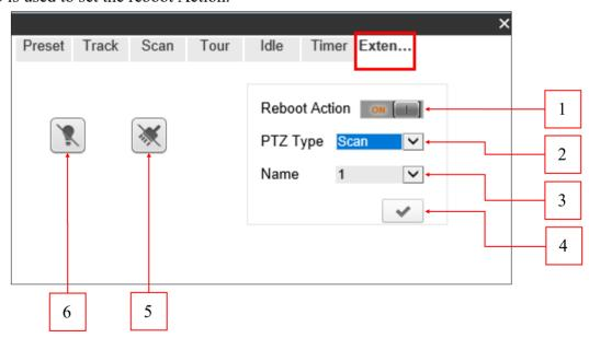
The *on/off* button (1) is used to enable/disable reboot action.
