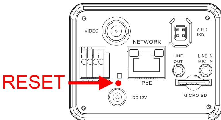
In the NVIP-5DN7000C-1P reset button is located as depicted below. Non metal, thin object (e.g. match) is recommended for pushing it.
