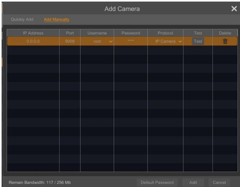
This menu allows you to manually create a camera in the system by entering the IP address of the camera, data port, user name and password.
