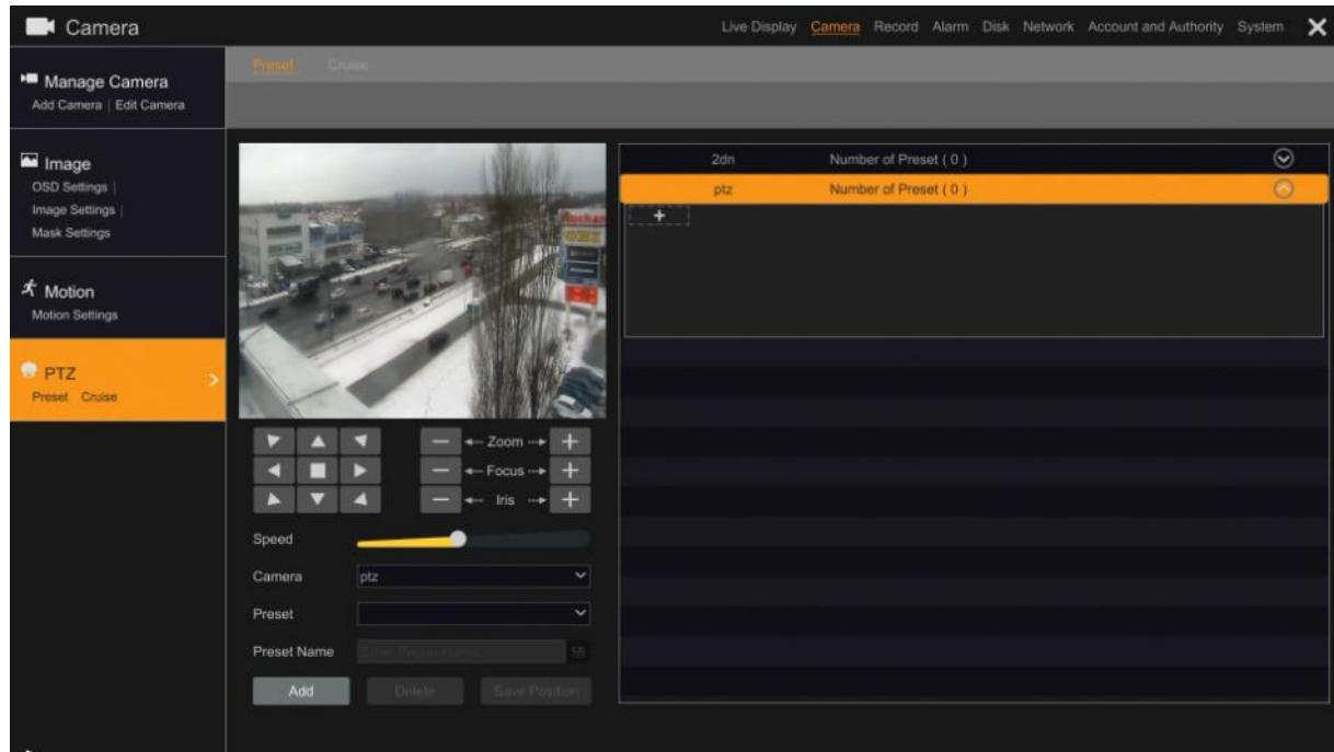
Using the control keys, select the position of the camera and press the ADD button. In the CAMERA you can change the point name and then press OK to add the point.
