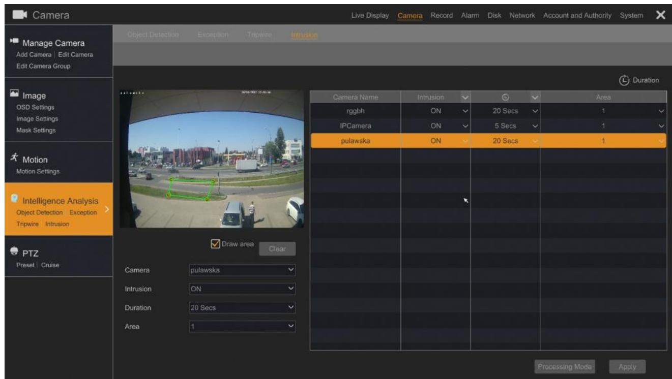
To designate the area check the DRAW AREA field and mark the zone using up to 6 points. To place the points press the left mouse button on the preview screen. Try to place the zone in the center of the image to make it easier for the camera to detect the object.
