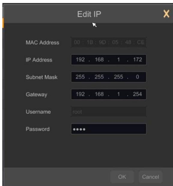
In EDIT IP window you can modify in IP ADDRESS, SUBNET MASK and GATEWAY fields. Press OK button to modify IP address for the selected camera.
