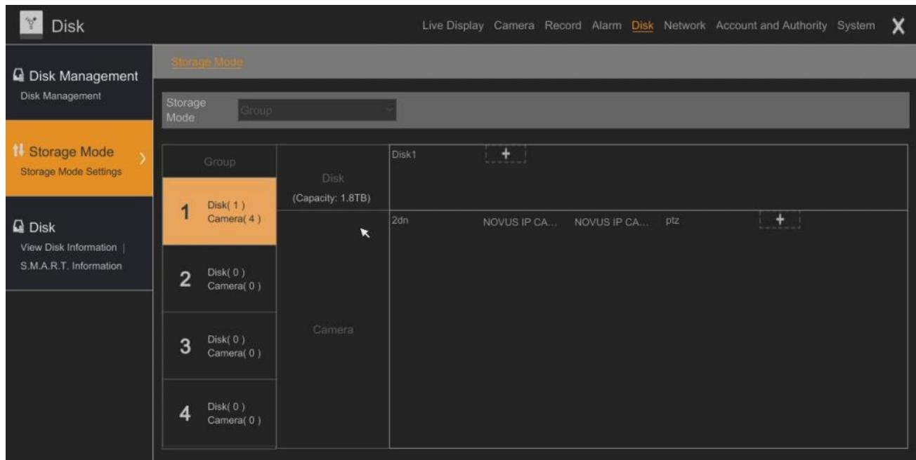
This menu allows you to create disk groups and cameras allocation to groups. This allows you to separate the recording cameras on each disk. (For NVR-6332-H2 and NVR-6332P16-H4).
