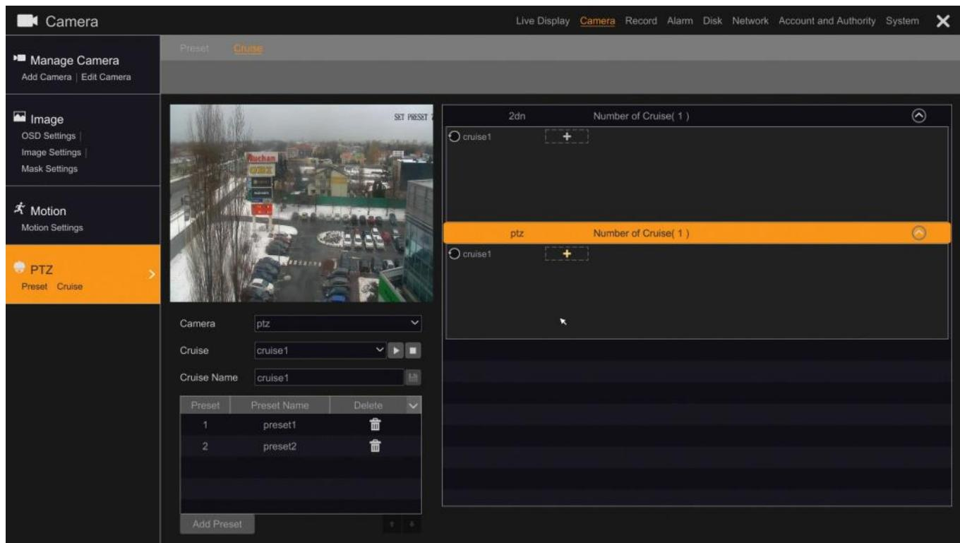
For the camera selected in the CAMERA, you can create a route consisting of (presets) defined in the menu PRESET. To add a point to the route, press ADD PRESET and select preset from PRESET NAME. Then select time for holding in chosen preset from TIME field and press OK to save the preset. Add few presets to create a cruise and then press floppy disk button to save the settings.
