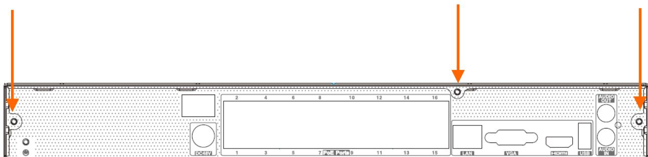
After cover removing, mount the disk or disks using mounting screws (4 pieces on the disc), then connect the power cord and signal cable.
