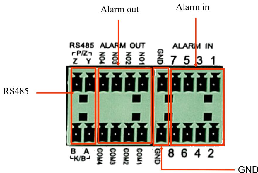
Example of connecting alarm output no. 1, follow the drawing below:
