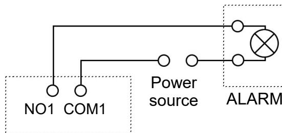
Example of sensor connection to alarm input 1.
