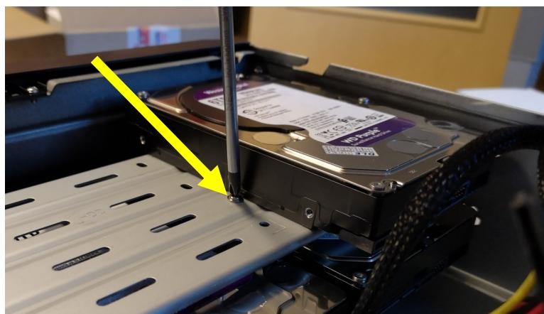
Mounted rails with disks should be secured by screwing out screws to the side of the housing.
