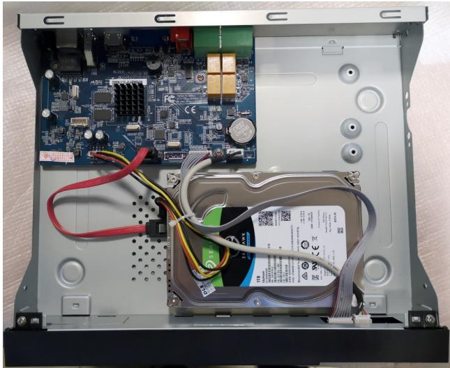
After connecting the hard drive mount the cover start the NVR to check and format the hard drive.
